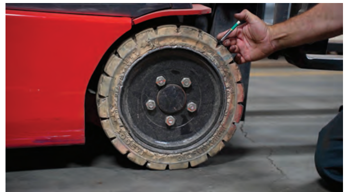
Using a tread depth gauge to determine how much tread is left.
