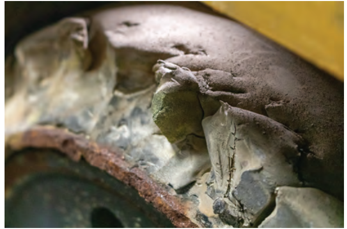
Tires with chunking decrease the stability of a forklift and can contribute to a tip-over accident.
