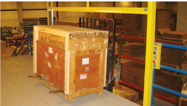
Vertical lift gate
