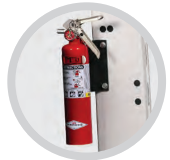
• Overhead Guard-Mounted Fire Extinguisher
